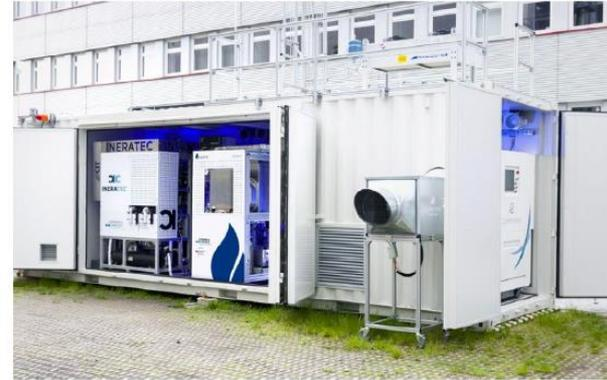
applications. The project, called C2 Fuels is deploying a small solid oxide system, with electrical capacity in the single-digit kW, in Dunkirk, France.<sup>49</sup>
