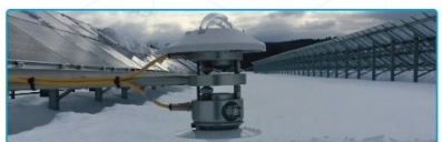
Figure 2. Images of irradiance sensors at three field sites: (clockwise from top left) POA pyranometer and reference cells on baseline system in Vermont, USA; POA pyranometer and PV-modules in Halle, Germany; GHI and DNI sensors in Köthen, Germany; irradiance sensors in Florianopolis, Brazil; (above) albedometer in Vermont.
