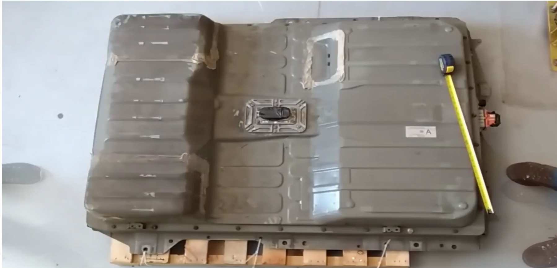
25 kWh Nissan Leaf Li-ion battery pack being repurposed for second life, stationary applications at the UFSC Solar Energy Research Laboratory
