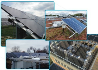
Figure 2. Images of irradiance sensors at three field sites: (clockwise from top left) POA pyranometer and reference cells on baseline system in Vermont, USA; POA pyranometer and PV-modules in Halle, Germany; GHI and DNI sensors in Köthen, Germany; irradiance sensors in Florianopolis, Brazil; (above) albedometer in Vermont.
