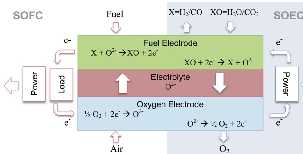
Fig. 1. Operating RSOFC principles: SOFC and SOEC modes.
