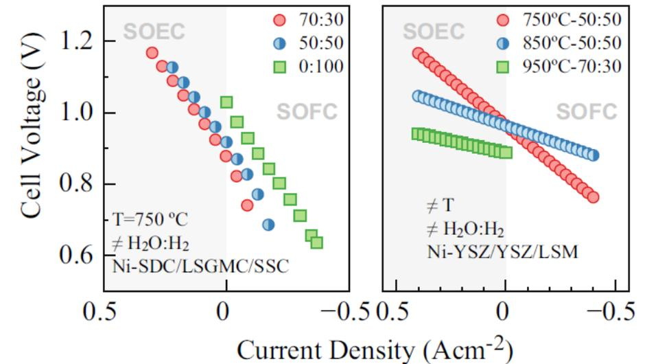
Fig. 3. Current density ( $J$ ) vs. voltage ( $V$ ) curves from different works [19,43–45]. Yttria-stabilized zirconia (YSZ), scandia-stabilized zirconia (ScSZ), samaria-doped ceria (SDC), samaria strontium cobalt (SSC), lanthanum strontium gadolinium manganite cobaltite (LSGMC), lanthanum strontium manganite (LSM).
