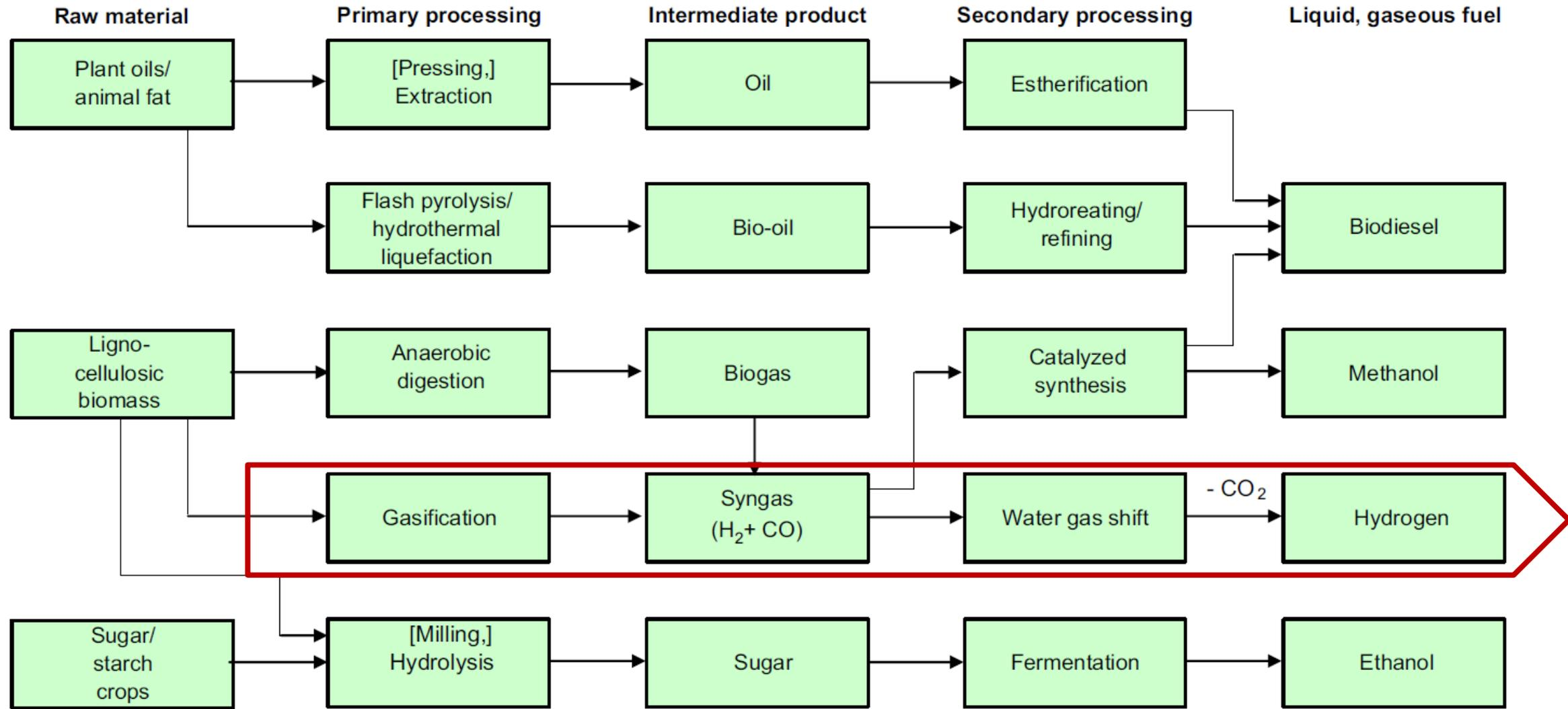
Fig. 3 – Overview of typical processing routes to biofuels.
