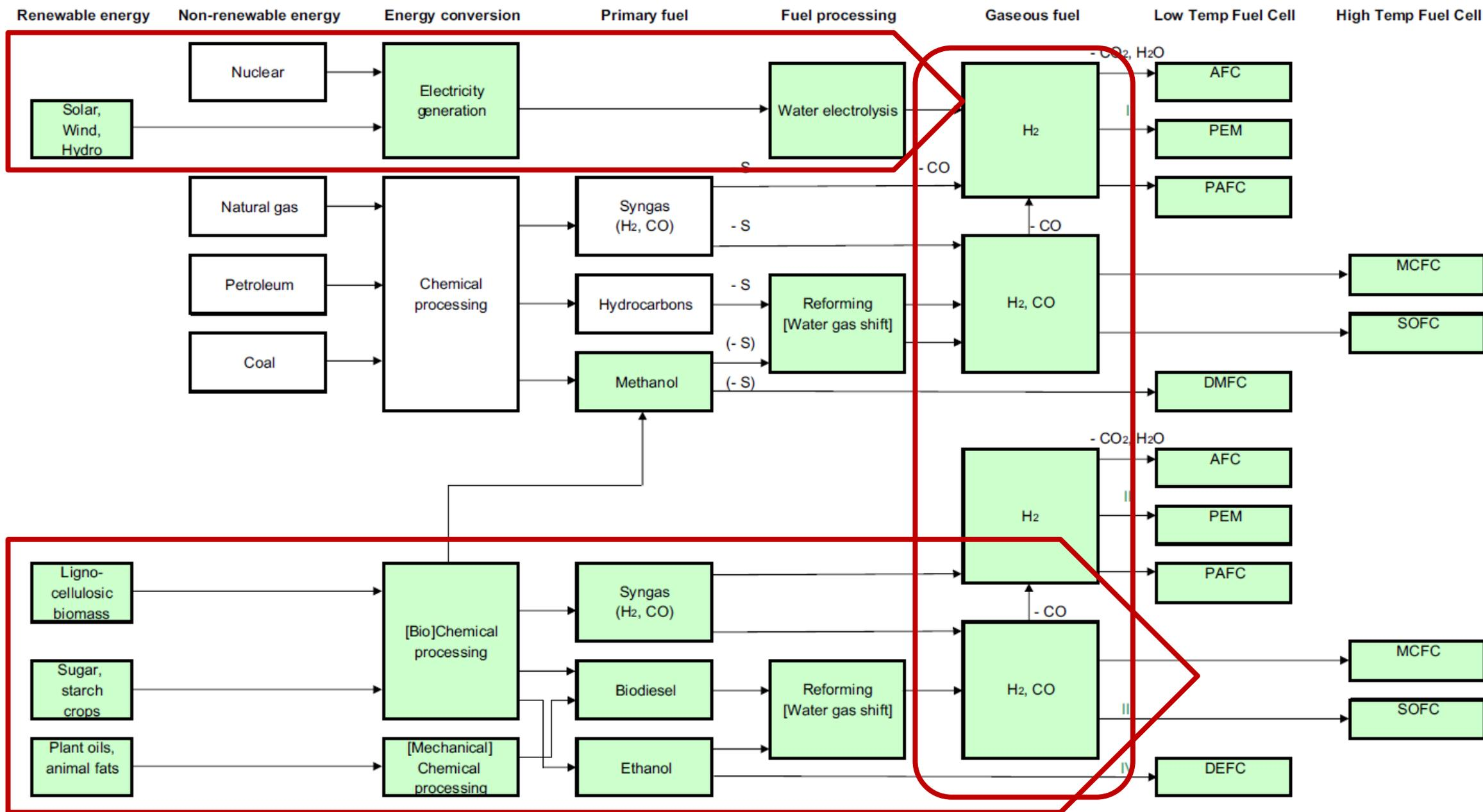
**Fig. 1 – Renewable and non-renewable energy sources, fuel processing and fuel cell technologies. The terms and abbreviations are explained throughout the text.**
